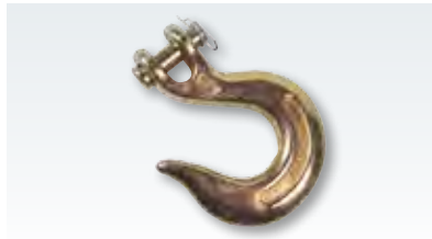
3/8 in. (10 mm) Alloy Clevis Slip Hook (#21006) 3-3/4 in. wide by 3/4 in. (95 x 19 mm) deep grip.
