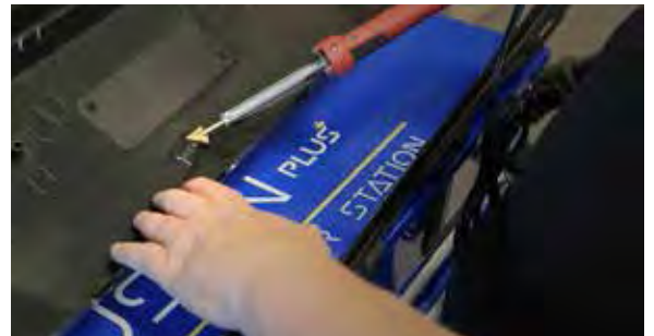
Fusion Plus accessories include smoothing iron for touching up final bead.
