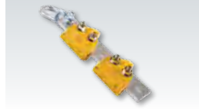
Frame Rack Unibody Clamp (#18062) Two pair of jaws with 12 in. (305 mm) draw bar with shackle and oval loop.
