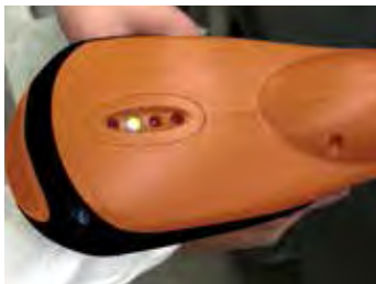
4 LEDs indicate state of device. Yellow (shown) means in use.
