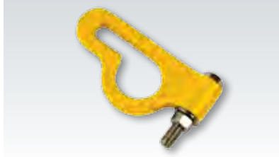
Numerous Angle Puller (#18022) Use with 3/8 in. (10 mm) chain to pull from any angle. Put the bolt through a 1/2 in. (13 mm) hole to pull. Use with #14404 Strut Tower Multi-Adapter.
