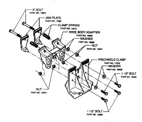
2. Install the pinchweld clamp onto the Pinchweld as usual . Proceed with the standard setup procedure as shown in the wedge clamp Training manual " Setting up the Anchoring system."
