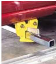
**2** Slide Anchoring Bars through EZE Tie-Down Sill Clamps. Make sure Anchoring Bars are centered. Insert Wedges into EZE Tie-Down Sill Clamps. Secure using a 3 lb. hammer.
