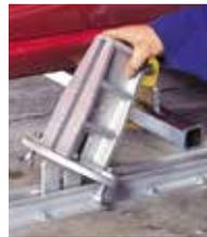
**4** Place EZE Tie-Down Anchoring Towers over Rail Dogs and slide Anchoring Towers up to Anchoring Bars.
