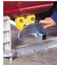
**5** Insert Crossbar Lock Plate through EZE Tie-Down Anchoring Towers and over Anchoring Bars.
