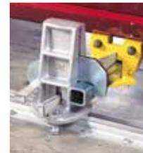
**6** Drive Wedges into Crossbar Lock Plate and EZE Tie-Down Anchoring Towers. You're ready to go!
