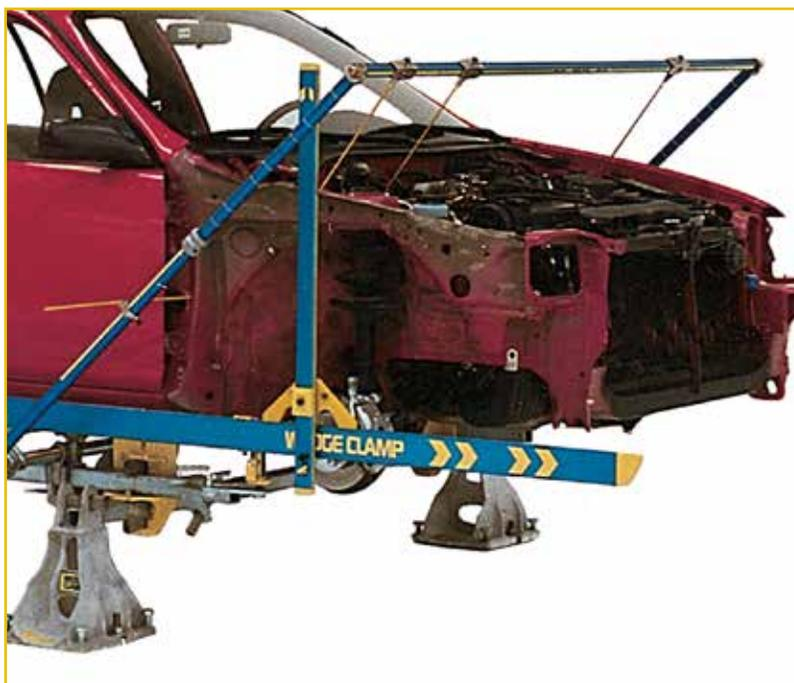
*The Length and Height accessory is used with the Pivot Measuring System to give you three-dimensional spec book measuring anywhere on the vehicle. This system is especially useful in repairs of heavily hit vehicles where large sections are being repaired or replaced.*
