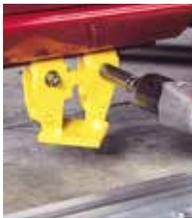
**1** Center vehicle between Anchoring Rails. Install the EZE Tie-Down Sill Clamps at the front and rear torque box areas of the vehicle.
