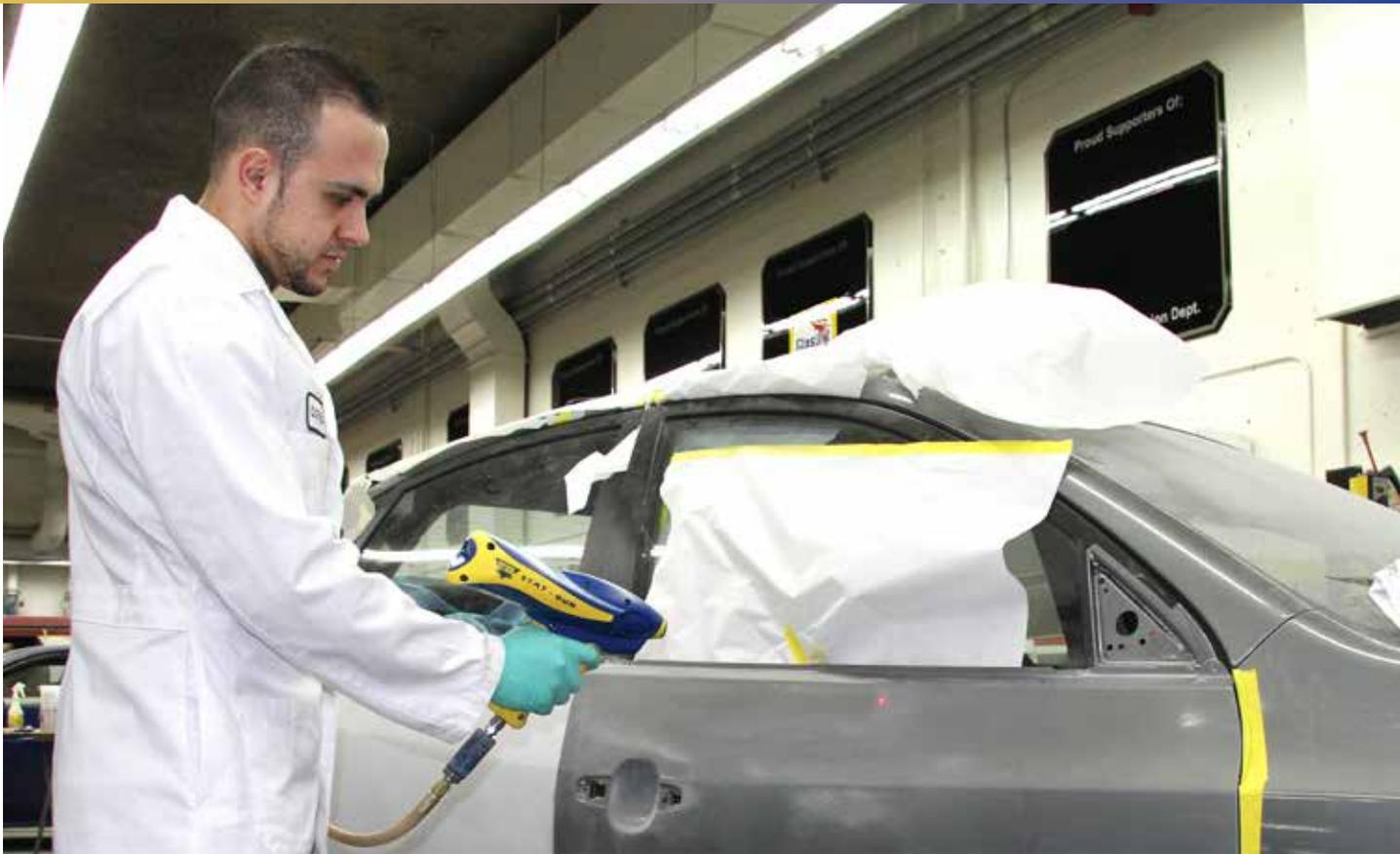
**Anti-static device's microprocessors and tungsten emitters** deliver a powerful, laser-guided ion stream that electrically neutralizes surfaces. Simply use instead of regular blowgun. Battery power eliminates cumbersome cable, lasts up to 12 hours of continuous use.
