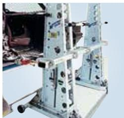
**Back Brace (#20600)** An optional back brace joins two Monocoque Towers together, allowing additional pulls to be made between them. Includes 6 ft. (1.83 m) Bracing Beam, Mounting Brackets (2), Pulling Brackets (2), Locking Wedges (4), 5 ft. (1.52 m) Lifting Beam with Support Chain and Lock, 5 ft. (1.52 m) Plated Alloy 5/6 in. Support and Chain, and 2 Chain Pulleys.
