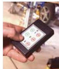
**Remote control (optional)** lets you control two separate pulling towers with single device for double independent pulls.
