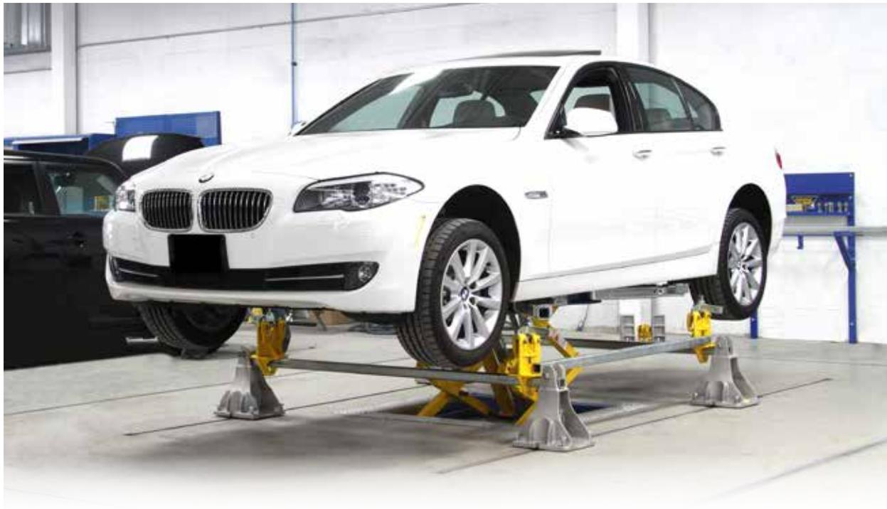
Designed for medium-size jobs, the Chainless Anchoring System ties to compact rails mounted either on top of the floor or embedded flush into the concrete. The low-weight aluminum stands allow effortless set up.
