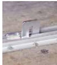
**3** Slide Rail Dogs into place on Anchoring Rails (front and rear).
