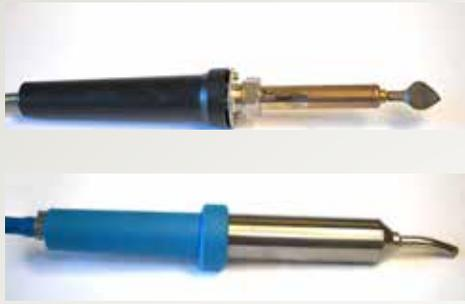
**NitroWeld 650 system** comes with 4 nozzles, including tacking nozzle (top) and round nozzle.
