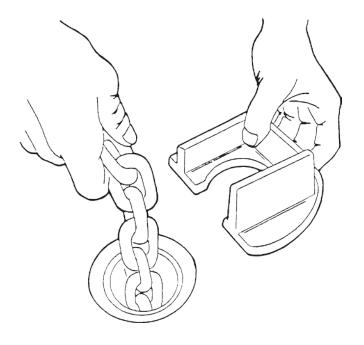
Holding the chain straight, select a link and a height position on the Press Spacer that results in the Press Handle being up from the floor at approximately 60.
