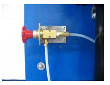
Safety lock release (red) button mounted at the Control Box
