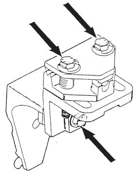
For certain models with the pinchweld displaced far outboard it may be necessary to use the spacer and longer bolt supplied with the kit to move the adjusting bracket and horizontal jaw further outboard. (See drawing below).
