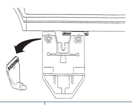
Loosen the bolts on the bracket. (See drawing below)
