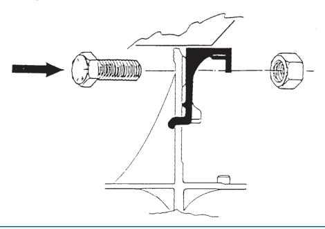
First, tighten the bolt on the clamp. (See drawing below)
