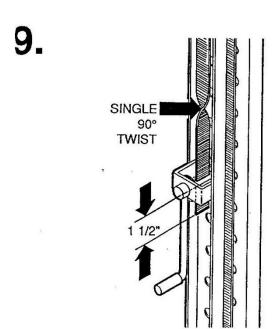
Turn the strap so that it has a single 90° twist, and thread 1 1/2 inches (4 cm) through the slot of the crank handle as shown.
