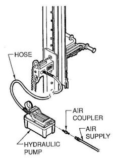
Attach the hydraulic pump hose to the hydraulic ram as shown.
