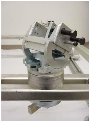
Figure 2: Close-Up of Swivel Base Assembly
