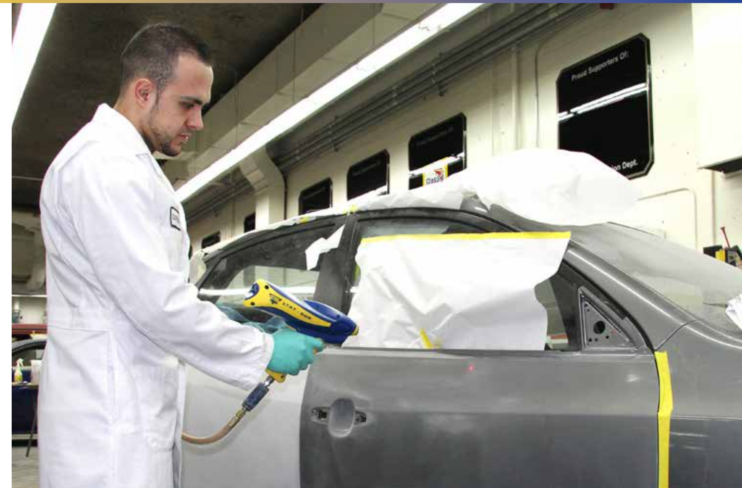
Stat-Gun's microprocessors and tungsten emitters deliver a powerful, laser-guided ion stream that electrically neutralizes surfaces. Simply use instead of regular blowgun. Battery power eliminates cumbersome cable, lasts up to 12 hours of continuous use.
