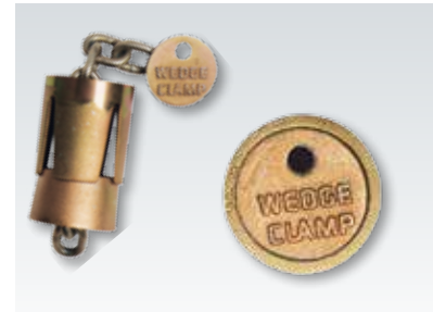
Floor Anchoring Pot (#17302) 3 1/2 in. (89 mm) cast iron construction. Precision machined for perfect fit. Zinc plated for corrosion resistance. Unique design facilitates replacing damaged chain.
