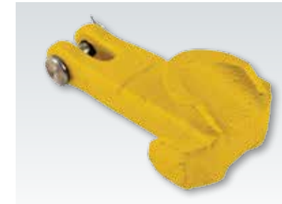
Hole Plug (#14116) 4-way anchoring tool for unlimited body and frame hook-up in existing holes. Attaches directly to 3/8 in. (10 mm) chain.
