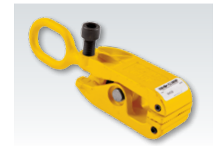
Flash Clamp (#18414) 5-ton spring-loaded clamp with pivoting heads for secure grip on uneven surfaces. Heat-treated jaw casting for longevity and replaceable teeth. Also available in 3-ton and 7-ton.
