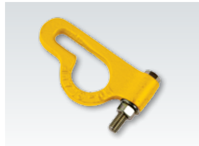
Numerous Angle Puller (#18022) Use with 3/8 in. (10 mm) chain to pull from any angle. Put the bolt through a 1/2 in. (13 mm) hole to pull. Use with #14404 Multi-Adapter Plate.
