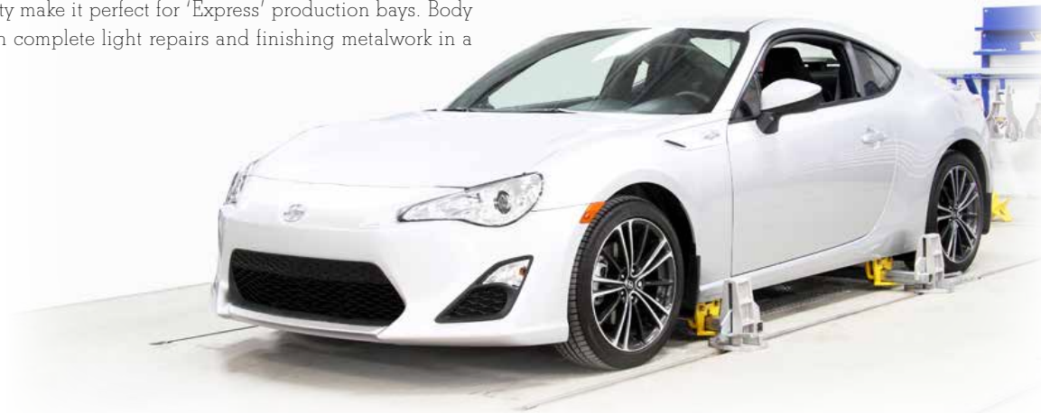
Vehicles are quickly mounted. No floor jack required.
