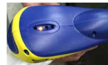
4 LEDs indicate state of device. Yellow (shown) means device is in use.
