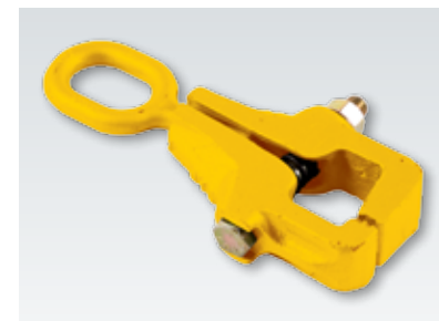
Box Clamp (#18404) Use to reach around flanges and other obstructions to grip hard-to-reach surfaces. Heat-treated jaws with aggressive tooth design for hard pulling power.
