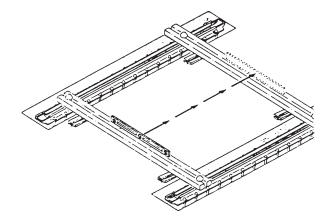
Be sure that the steel anchoring bars do not move during the concrete pouring process. It is advisable to place masking tape over the slots in the rails to prevent any concrete from falling into the slots during the pouring process. Remove the tape within three days of the concrete pouring to prevent the tape from hardening onto the rails.
