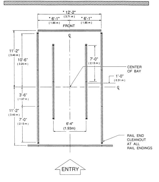
Note: \* Minimum width for the Monocoque Tower Pulley only. If using Eze Roller Pulling Towers use a minimum bay width of 14' (4.27 m).
