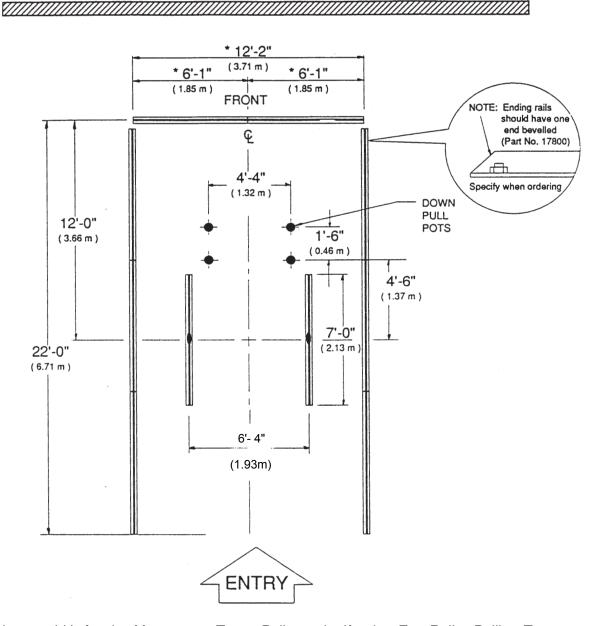
Note: \* Minimum width for the Monocoque Tower Pulley only. If using Eze Roller Pulling Towers use a minimum bay width of 14' (4.27 m).
