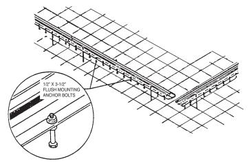
Suspend the wire mesh approximately 2" (51 mm) above the bottom of the concrete slab.
