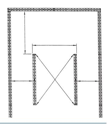
Use the rail as a template and drill a hole at each end of the rail on opposite sides of the rail. Insert an anchor bolt in each hole and tighten to hold the rail in position. Keep the drill straight while boring the holes.
