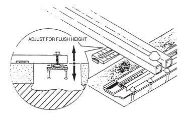
It is important that forward and rearward sets of steel anchoring bars are flat relative to each other. Using a carpenters level you can determine if the bars are level with each other.
