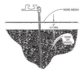
Allow the concrete to set for 23 days before any pulling is made on the rails. The tape used to cover the top of the rails should be removed within 3 days of the pouring process to prevent hardening of the tape on the rails.
