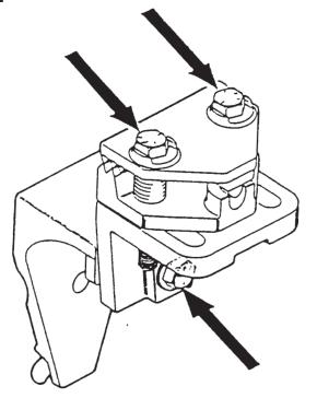
For certain models with the pinchweld displaced far outboard it may be necessary to use the spacer and longer bolt supplied with the kit to move the adjusting bracket and horizontal jaw further outboard. (See drawing below).
