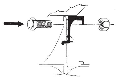
First, tighten the bolt on the clamp. (See drawing below)
