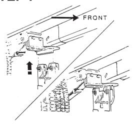
Install the pinchweld clamps onto the vertical flange on the brackets.
