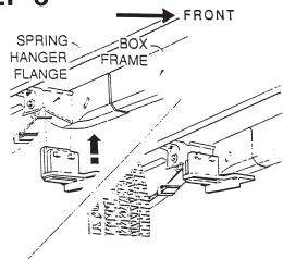
Position the rear brackets over the spring hanger flange as shown.
